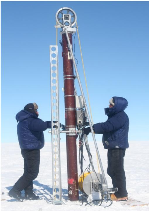
*A lightweight drill that can be separated into parts allows drilling both polar and high elevation glaciers.*
